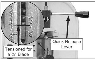
Figure 23. Example of tension applied for a %" blade.
